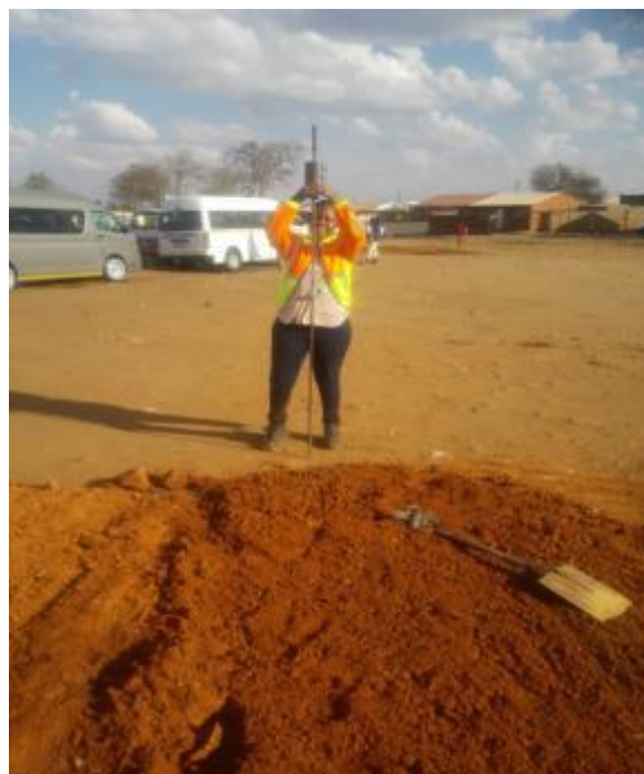
PIC B: DCP test underway
