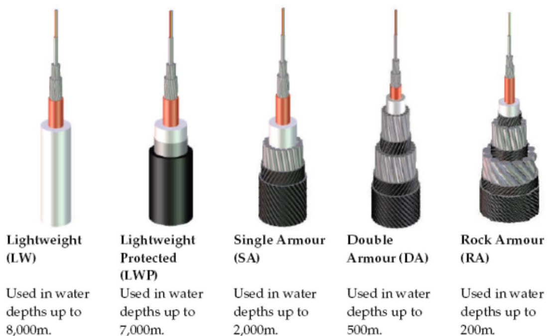
Plate 7 Cable armouring and operational depths
