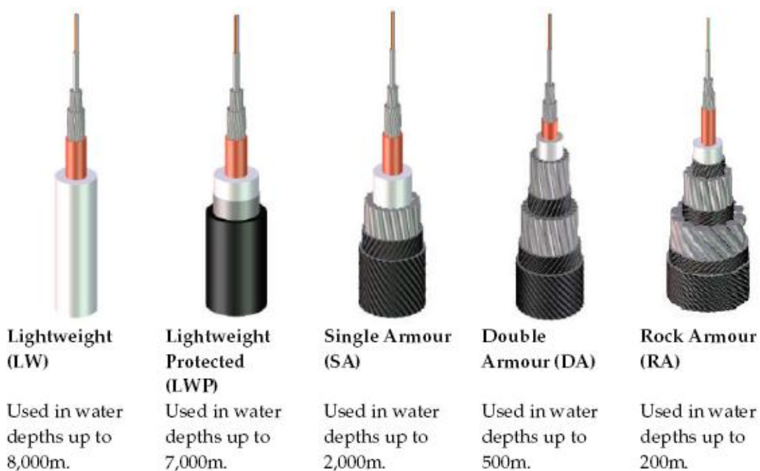
Plate 2 Cable armouring and operational depths
