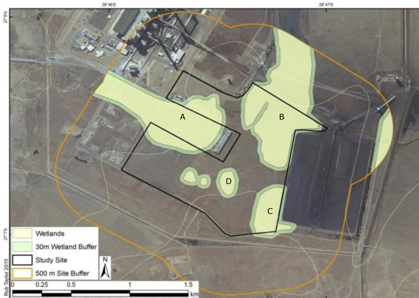
Figure 6.4: The wetlands and wetland buffers on the study site; A: the unchannelled valley-bottom wetland, B: a hillside seep draining northwards, C: a hillside seep draining south-eastwards, D: a cluster of hillside seeps draining north-westwards. All wetlands within a 500m buffer of the construction are prescribed by the DWS as relevant to the Water Use License application process.
