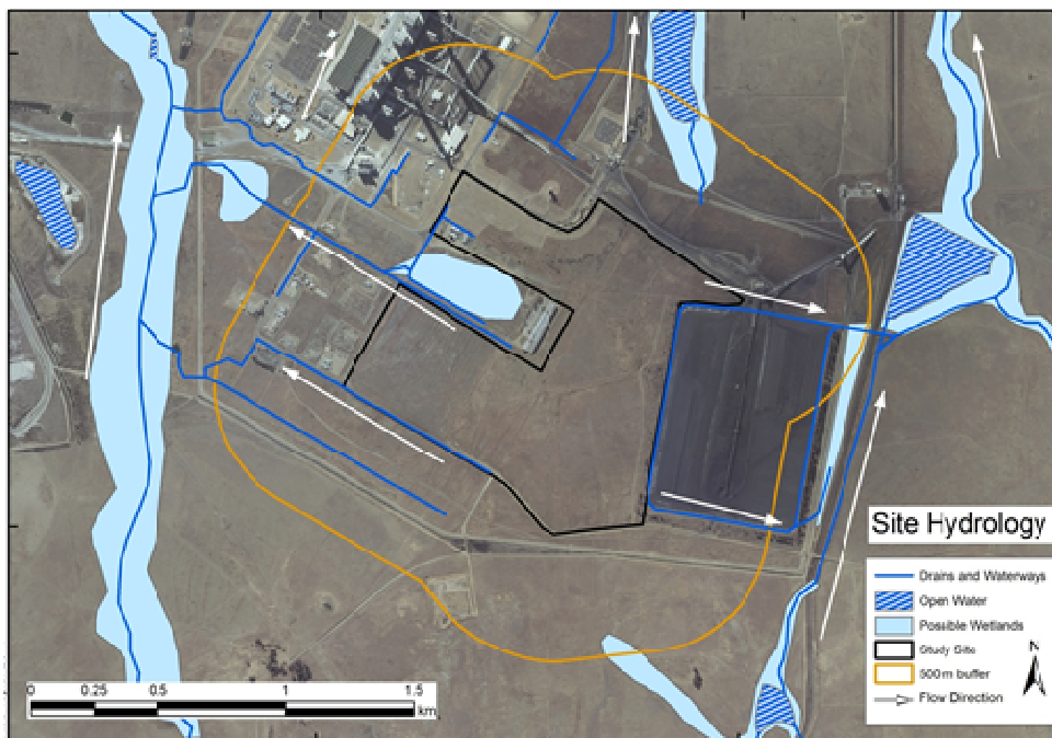
Figure 5.1: Site (black boundary) hydrology showing drains and waterways. The arrows indicating the direction of water flow.
