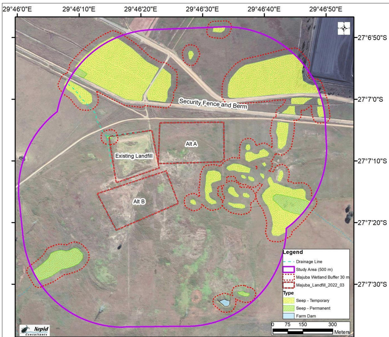
Figure 6.2: Delineation of aquatic ecosystems within the 500m regulated area of the development footprint alternatives
