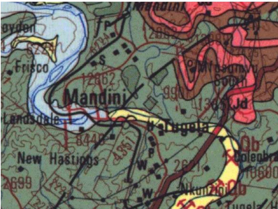
Figure 2: Approximate area of the proposed Mandeni Cemetery Development. Extract from the Durban 2930 Geological Map. According to this geological map, this development will be entirely on the Dwyka Group; however dolerite dykes may also be present.
