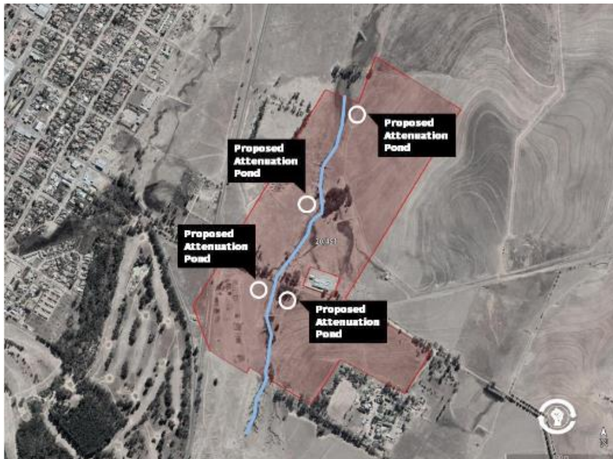
Figure 6: Regional Attenuation and Existing Stormwater Infrastructure
