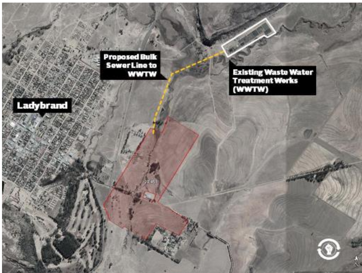
Figure 4: Proposed Sewer Connection Point(s)
