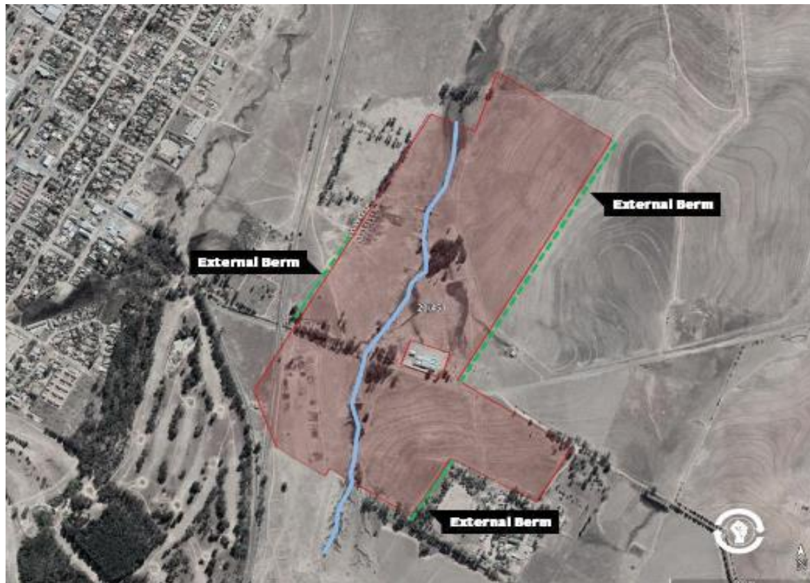
Figure 5: Proposed Stormwater Management from External Runoff
