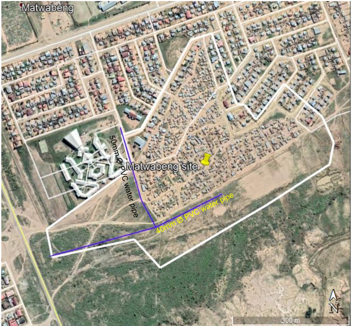
Figure 14 Existing water pipelines onsite
