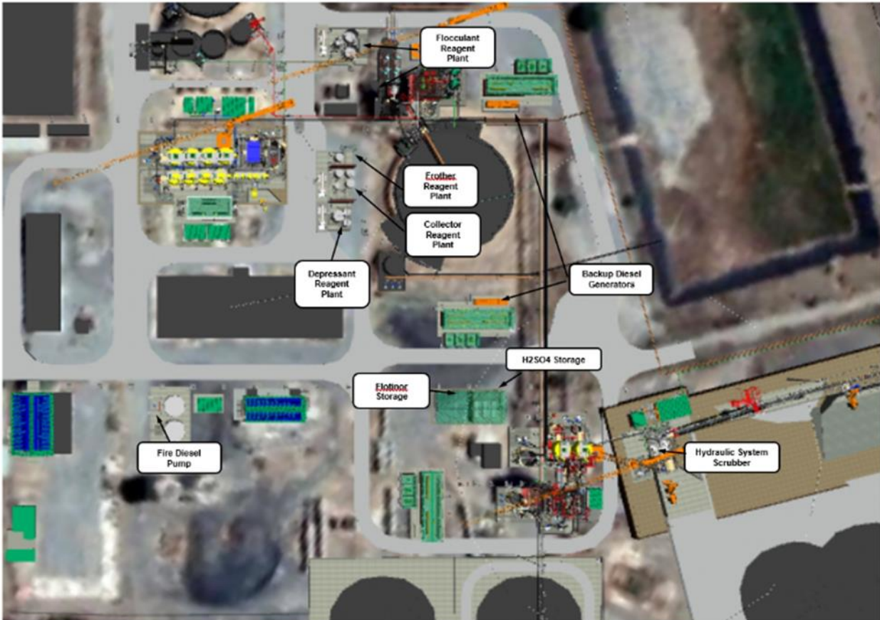
Figure 4-6: Dangerous Goods Storage Area
