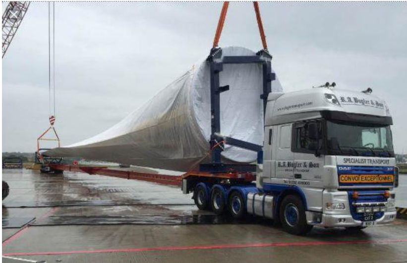
Figure 2-2: Example -Transport of Blades on extendible trailers
