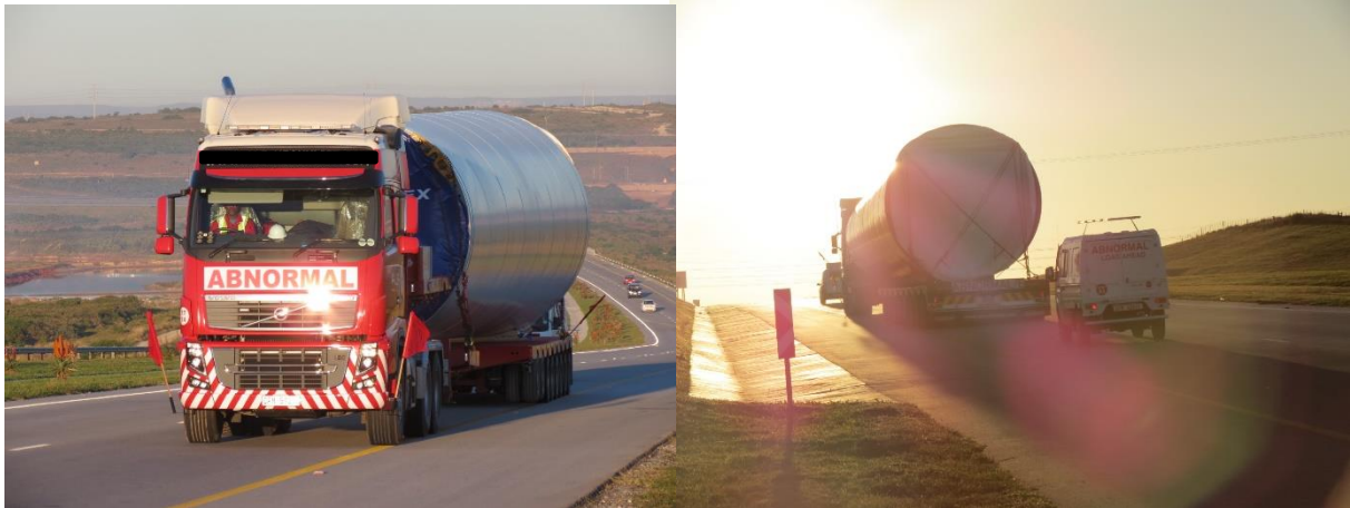
Figure 2-4: Example – Transportation of Tower Sections
