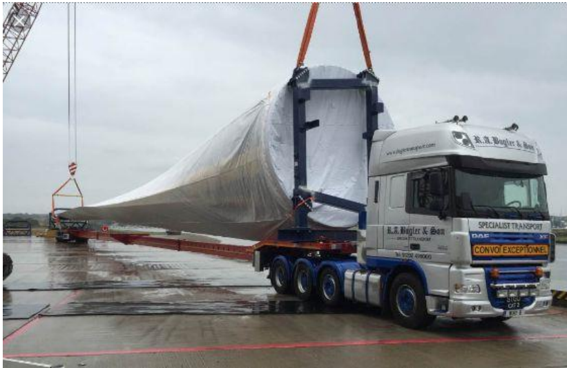
Figure 2-2: Example -Transport of Blades on extendible trailers
