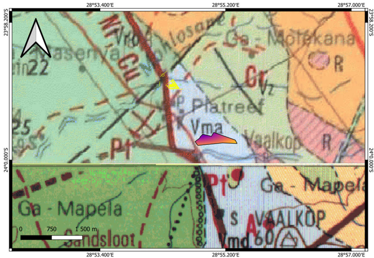
Figure 4: Extract of the 1:250 000 2328 Pietersburg (1985) Geological Map (Council of Geoscience, Pretoria) indicating the geology of the proposed development. The pre-assembly yard is indicated in yellow and the cable repair bay in multi-colours colours.
