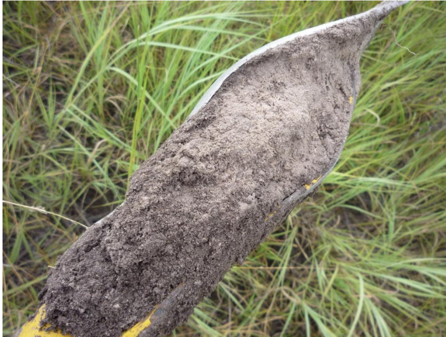
Figure 18 : Soil Sample Showing transition between the Othic A and underlying E horizon
