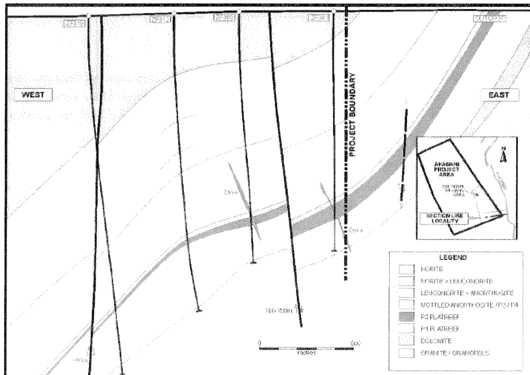
Figure 5: East-West Cross section through the south-eastern section of the project area, near the proposed bulk sampling shaft
