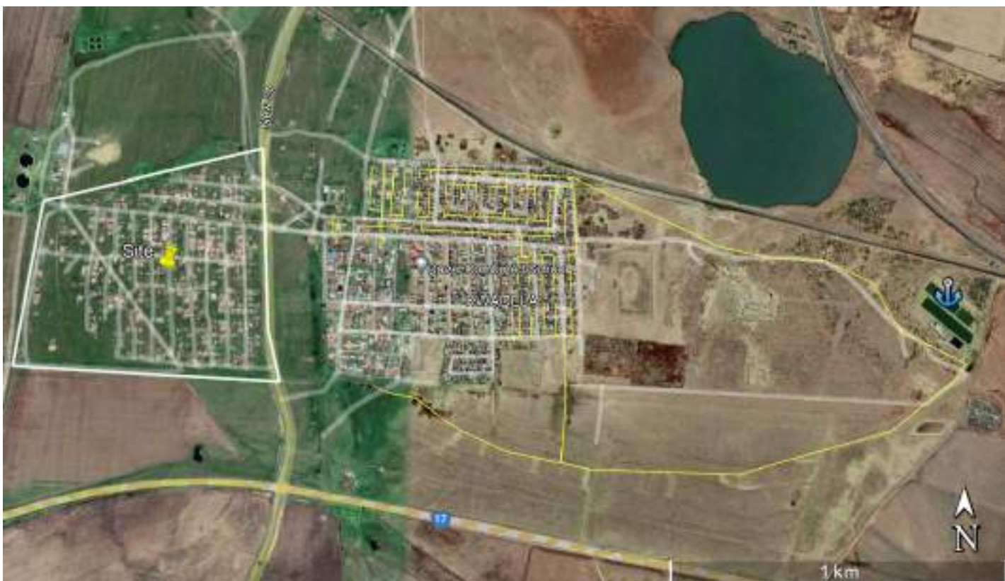
Figure 19 Sewer pipelines (yellow)
