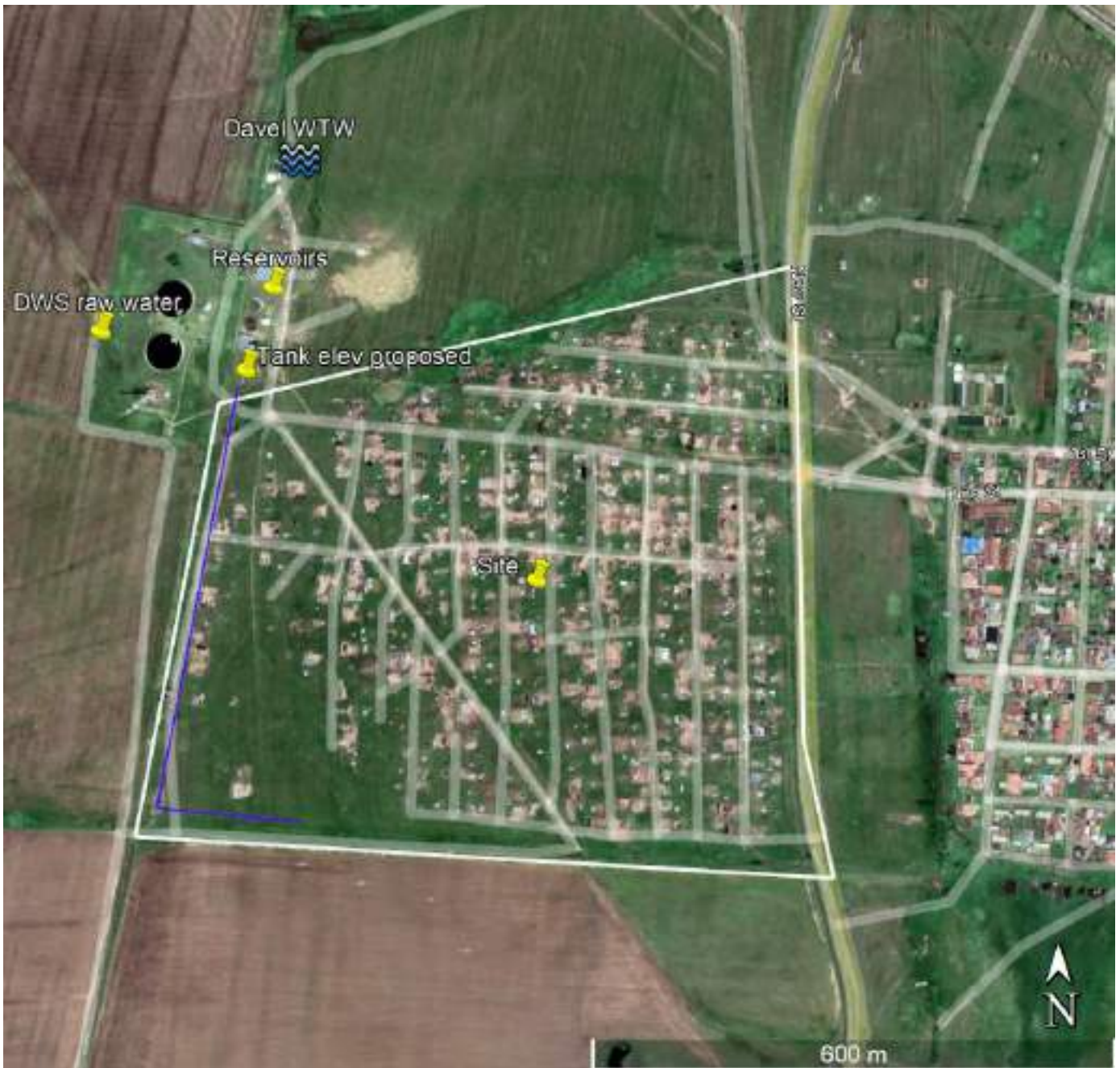
Figure 16 Proposed gravity delivery water pipeline (blue)
