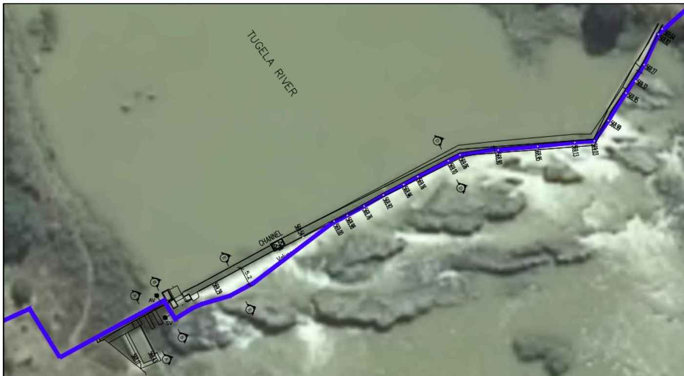
Figure 6: Engineers Drawing Showing the 200mm Pipeline Crossing Over the Thukela River (WC1), Highlighting the Sections of Pipeline Occurring Within the Watercourse. See Appendix A for the Full Design. Source: Civitech Engineers, 2020.
