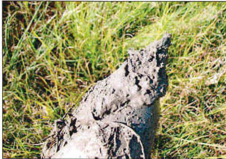
Photograph 1: An example of a soil with prolonged periods of saturation displaying a reduced matrix, as indicated by the grey colouration.
