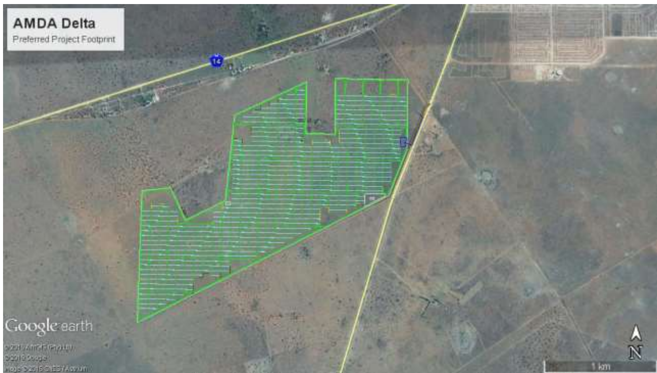
Figure 3: Proposed Facility layout showing access road and evacuation line
