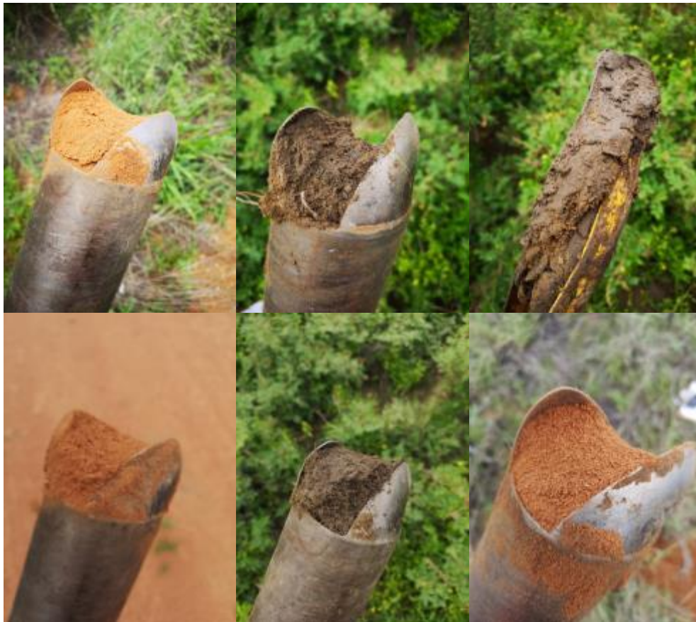
Figure 10-2: Example of structureless soils found site
