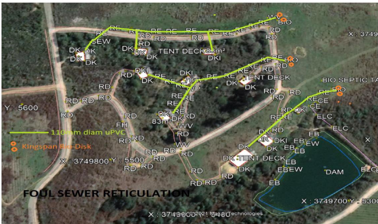
Figure 7.2 Sewer reticulation system at the Tented Camp site.
