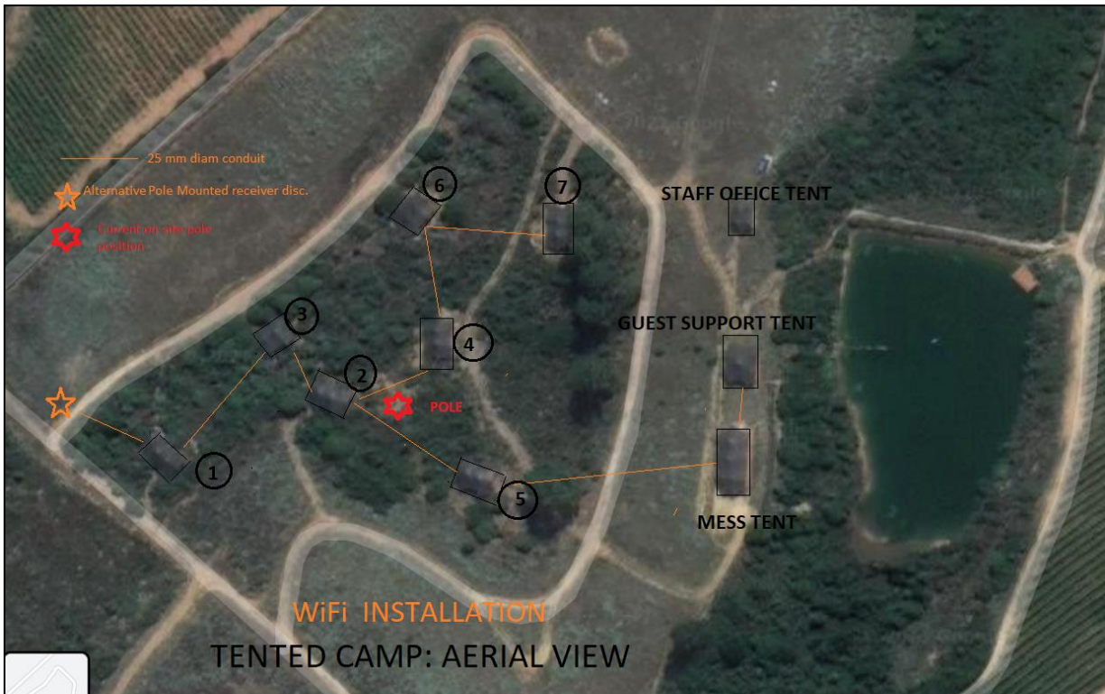
Figure 3: Internet cable installation (source: Hurworth, 2021)
