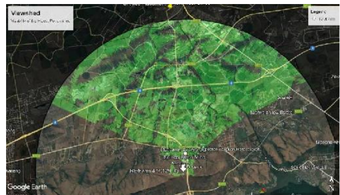
Figure 24 : Viewshed Calculation : Highest point mined would be visible from the areas in green.
