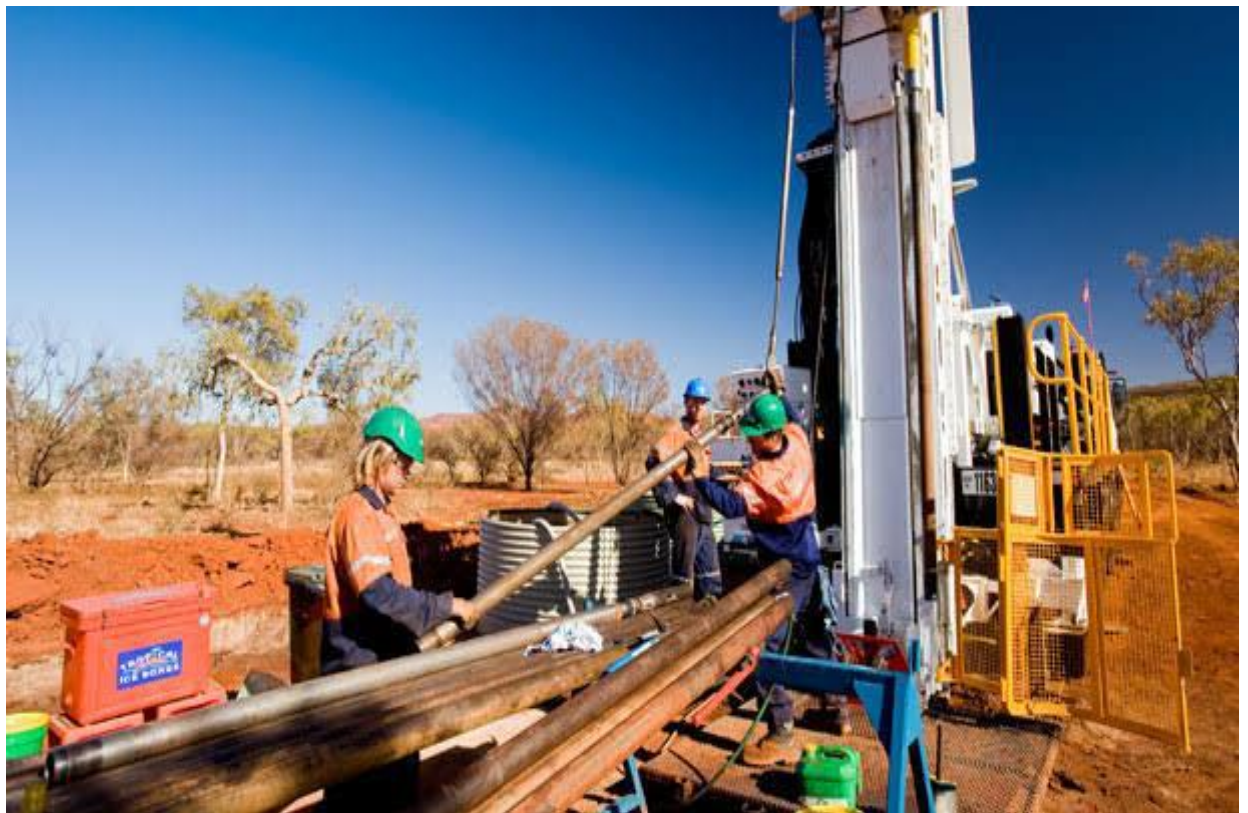
Figure 6: Typical example of Diamond Core drilling.
