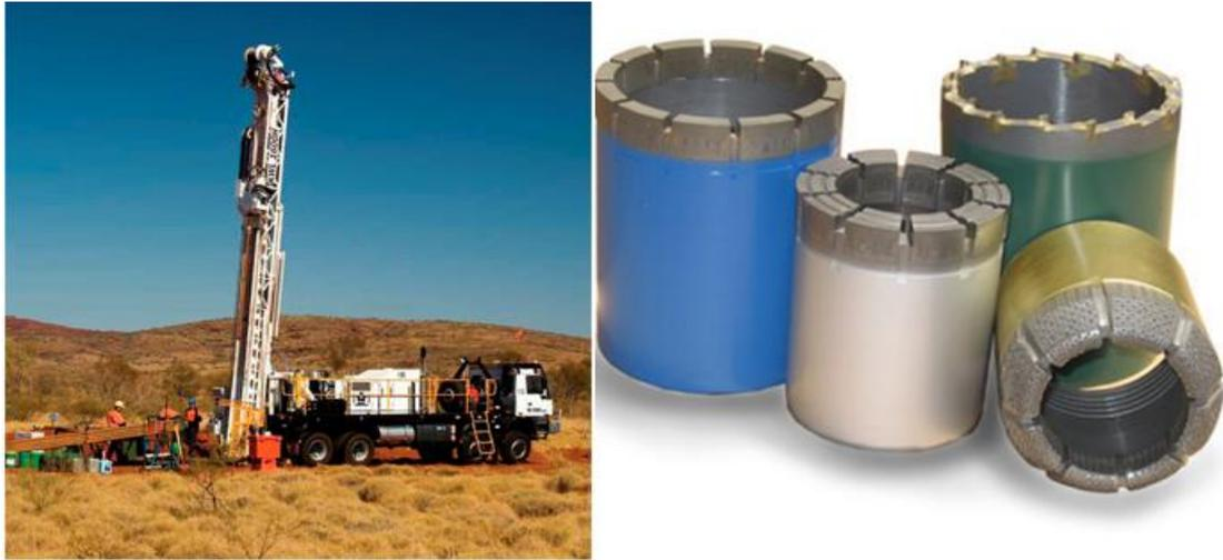
**Figure 6: Typical example of Diamond Core drill rig and drill bits.**
