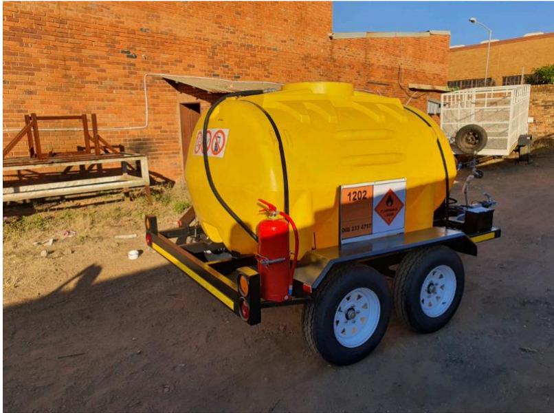
**Figure 10: Typical example of fuel transport to the site.**
