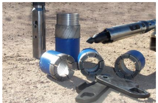
Figure 4: Typical example of Diamond Core drill rig and drill bits.
