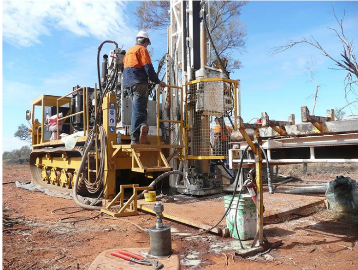
Figure 6: A Reverse Circulation drill rig.
