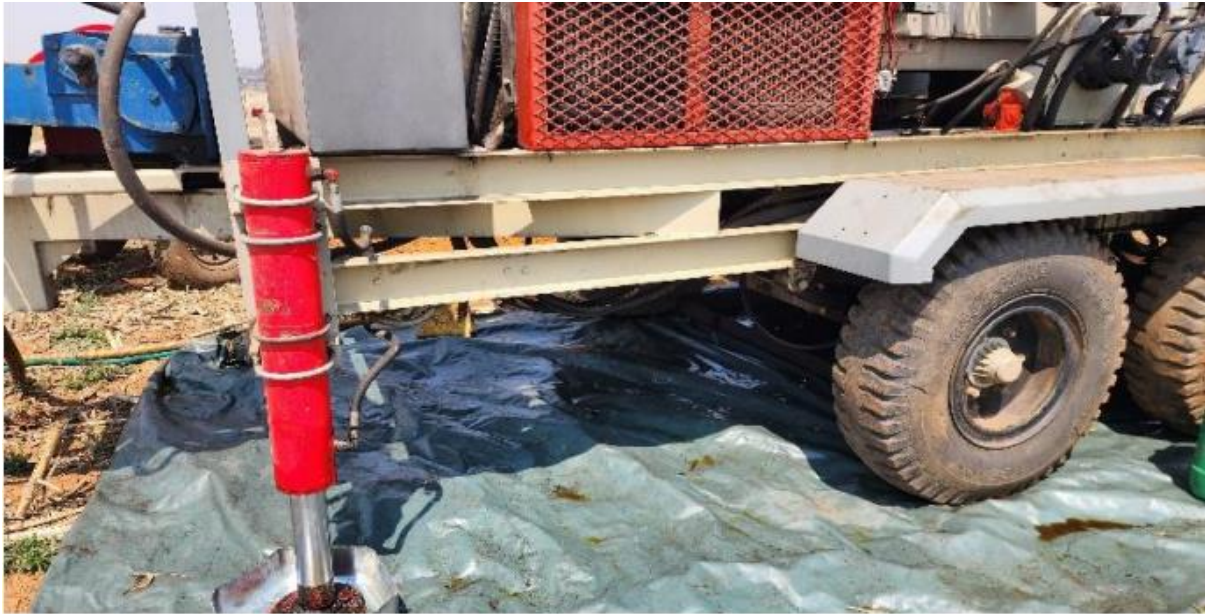
Figure 39: Drill truck placed on top of a lined plastic to prevent hydrocarbon leak.
