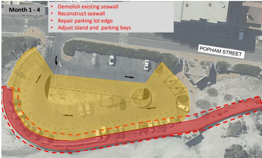
Figure 7.3: Construction of De Mist parking lot (4 months)
