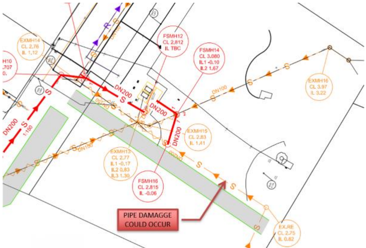
Figure 5.7: Option 2 – DN200 HDPE diversion at FSMH16
