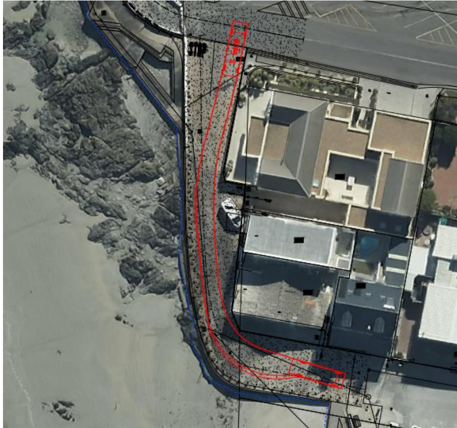
Figure 5.3: AutoTURN simulation of Pelegrini corner
