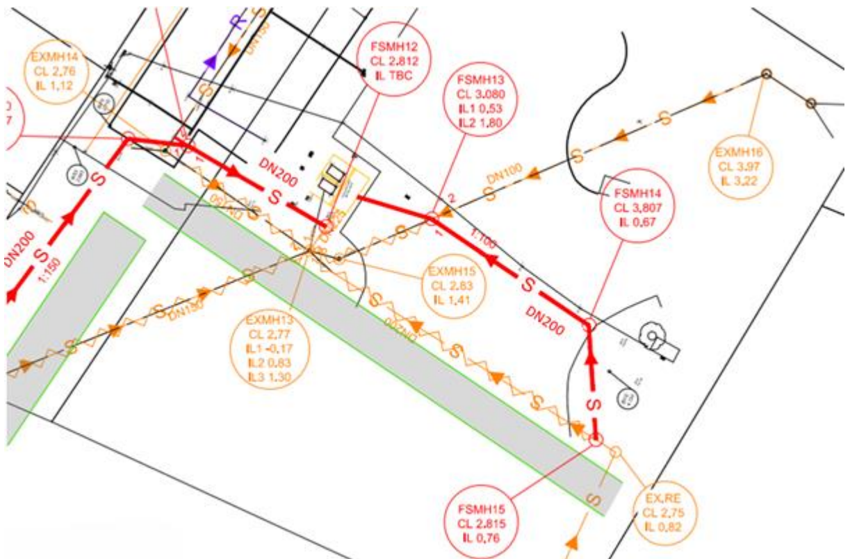
Figure 5.6: Option 1 – DN200 HDPE diversion at FSMH15
