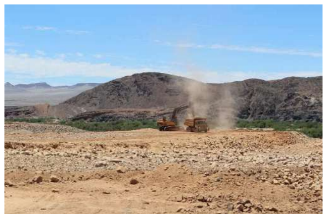
Photo 16: Excavator and dump truck used to extract gravels to load and haul to static processing plant
