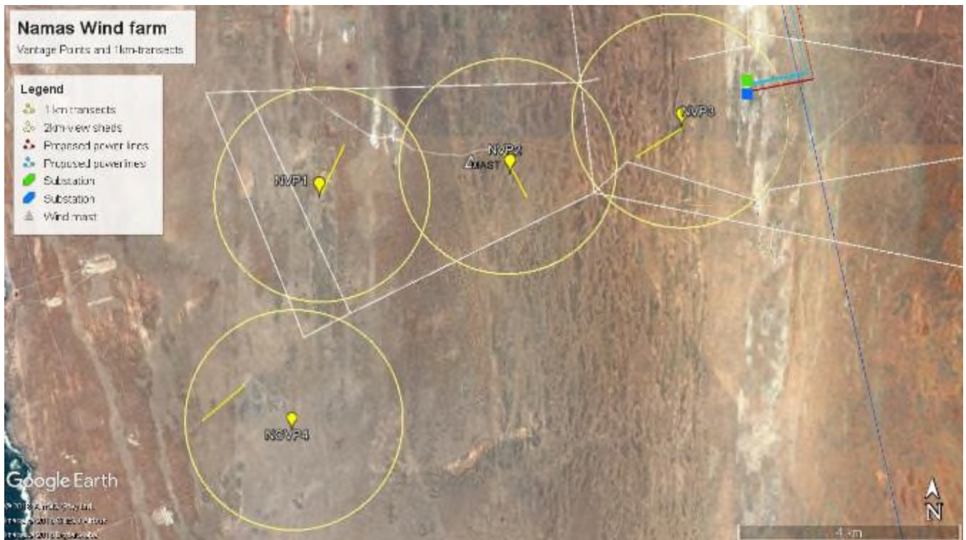
Figure 1: The 28-km 2 extent of the proposed Namas wind farm showing the boundary of the site (white polygon), the VP viewsheds of 2-km radius (yellow circles) and the 1-km transects in the WEF (yellow lines). A Control area with equivalent habitat and land-use was chosen to the south-west and surveyed simultaneously (NQVPA).
