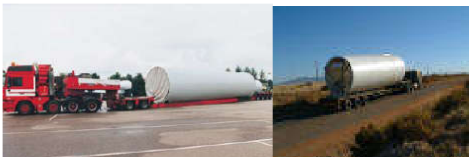
Figure 3-4: Transporting the Tower Sections (Source: Author's photograph)
