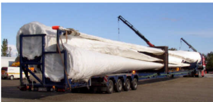
Figure 3-2: Example: 3 x 45 m Blades on extendible trailers 2
