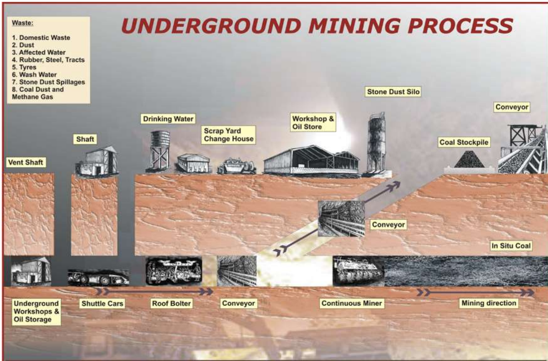
Figure 12: Underground Mining Process
