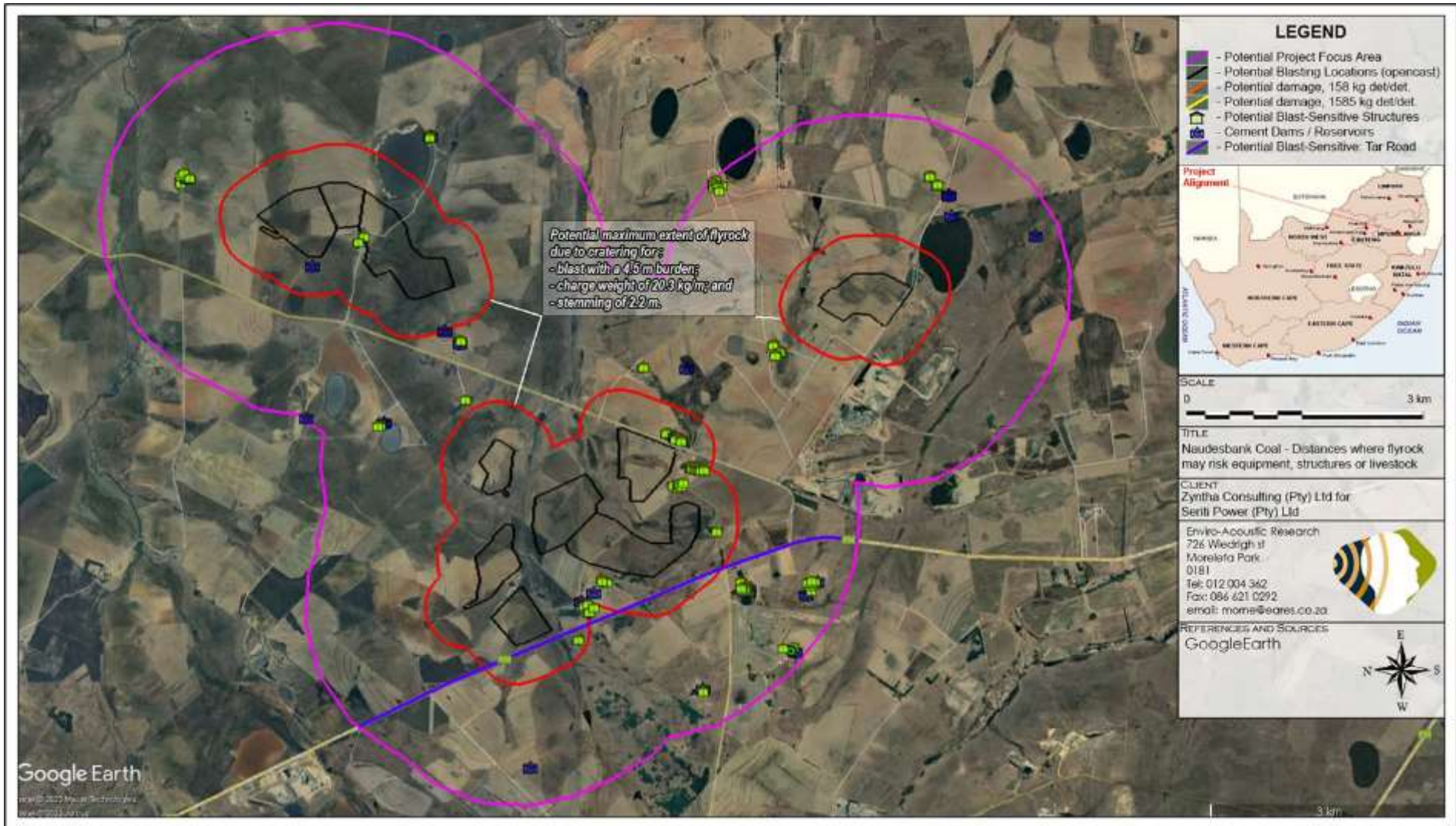
Figure 76: Blasting Sensitive Structures within 2 000 m of Opencast Areas
