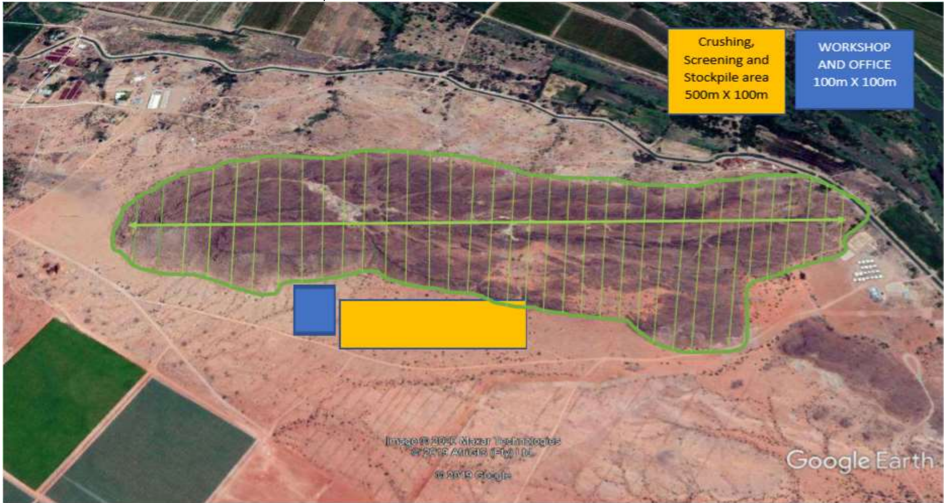
Figure 3. Schematic presentation of mine schedule of the production process. Mining will start from the middle of the deposit which sits in the form of a kopje and will continue in both directions in blocks which is not to scale on the sketch.
