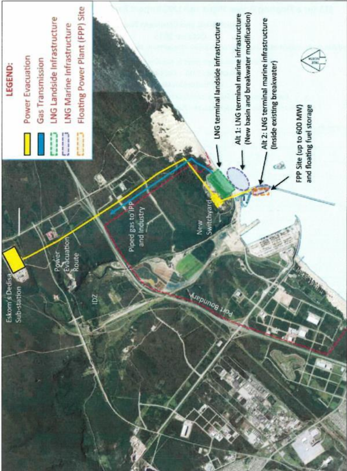
Figure 8: Proposed location for the LNG Import Facility in the Port of Ngqura
