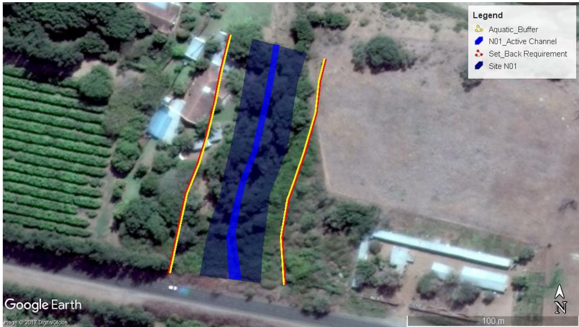
Figure 26: Delineation of the N01 Riparian site's active channel edge, aquatic requirement, riparian edge and then the final setback requirement
