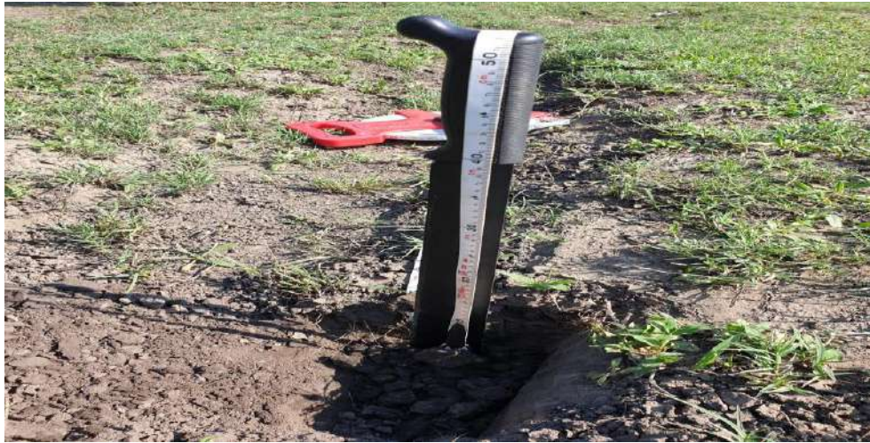
Figure 4.2.1: Indicator for soil sampling during field survey
