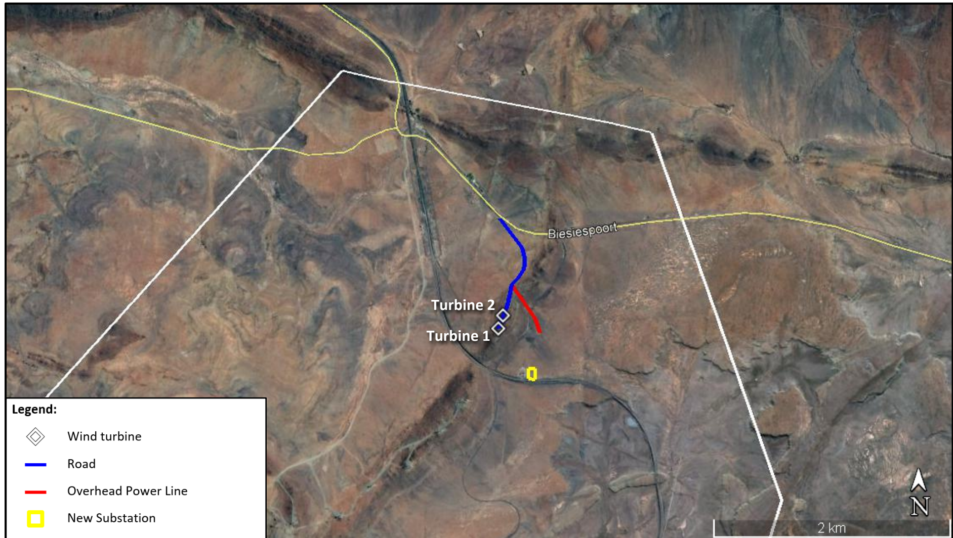
Figure 3: Layout for the proposed road, OHPL and two upgraded wind turbines, showing the Noblesfontein Site's Northern boundary, completed turbines to the South West, and the position of the proposed second substation adjacent to the existing authorised and constructed substation.
