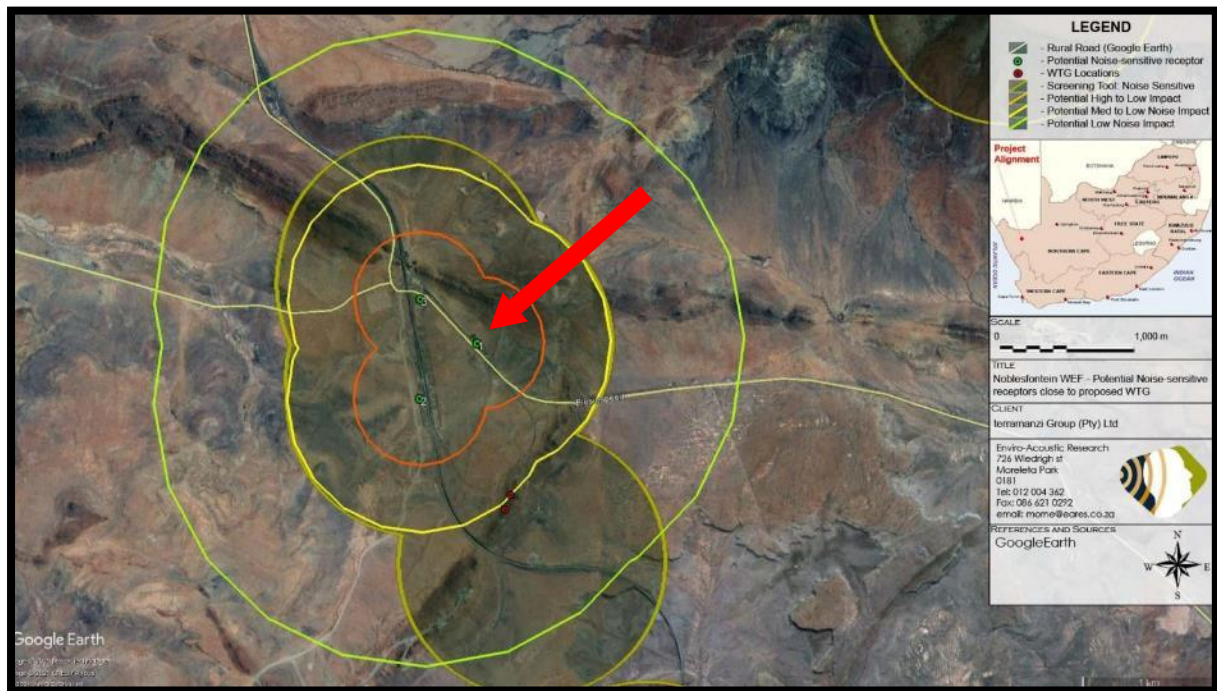
Figure 8.8: This figure shows the Potential Noise Sensitive Areas and identified receptors. Site Sensitivity Verification found that only a single occupied residential dwelling/receptor exists (Red Arrow).
