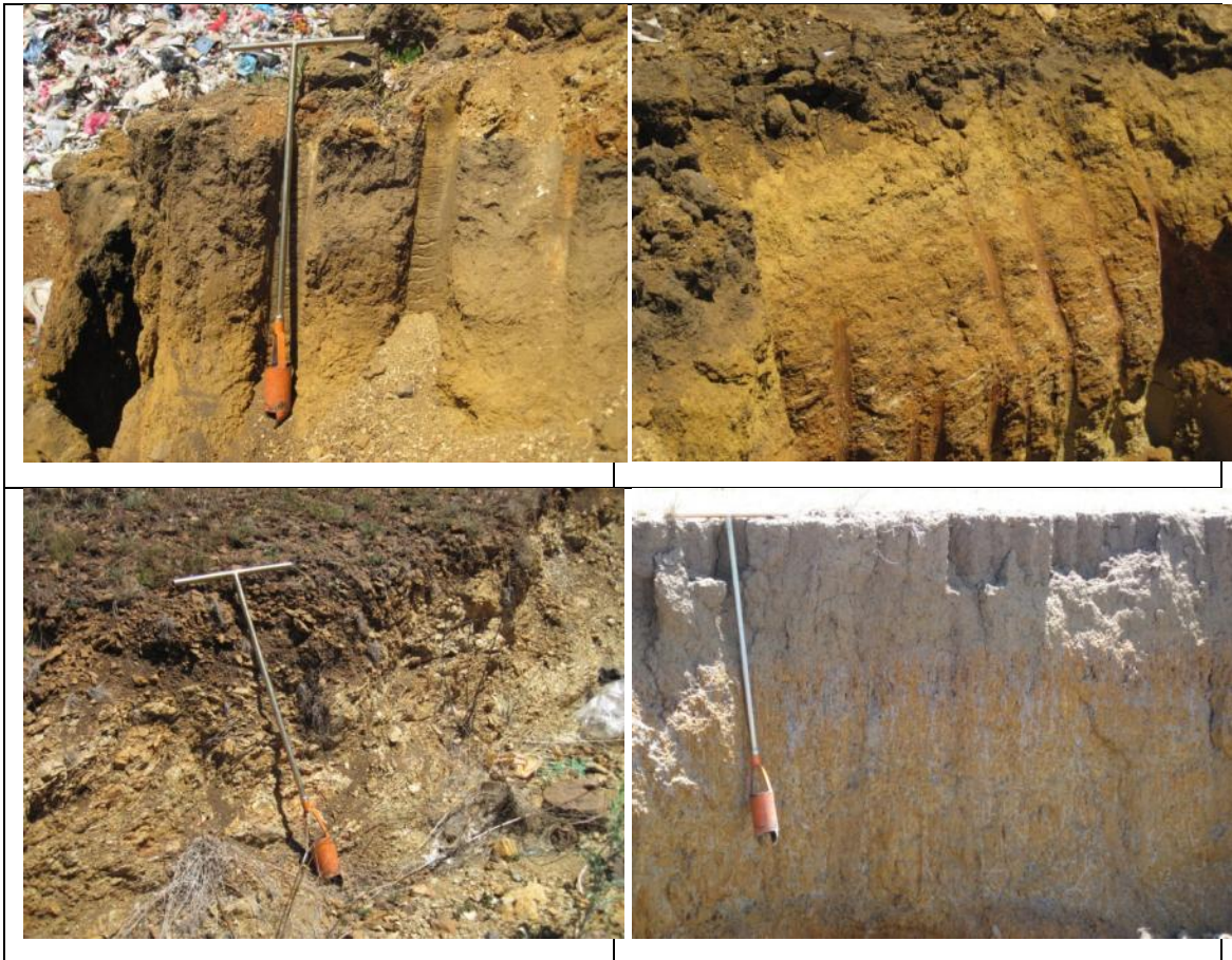
Figure 3: Illustrates soil profiles within the study area that lacked wetland features, such as mottling, gleying and spots of iron depletion (top row and bottom left), and distinct wetland features in the form of mottling within the top 0.5 m of the soil profile and gleying below that, as recorded on an exposed headcut profile that is eroding into a seep wetland, southeast of the landfill site (bottom right).
