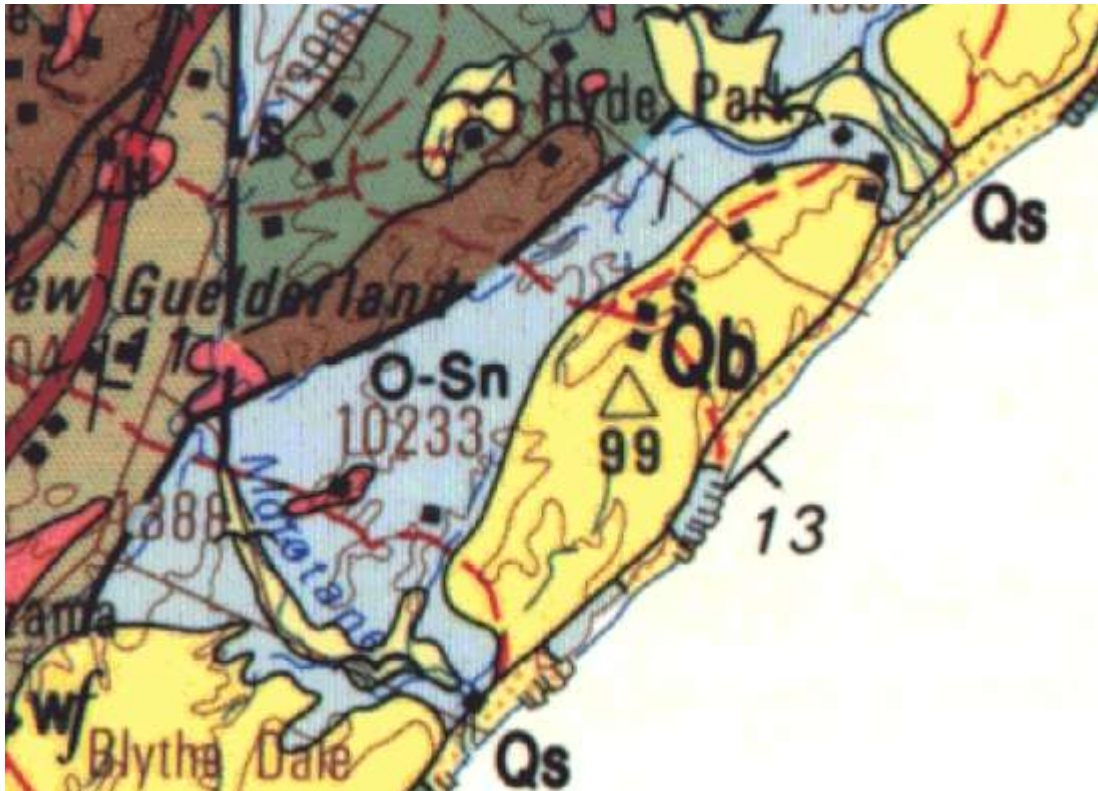
Figure 2: Approximate area of proposed Nonoti Beach Development Node. According to this extract from the Durban 2930 1:250 000 Geological map, the proposed footprint will overly mainly the Umkwelane Formation (Qb: yellow on map), although the Kosi Bay Formation (Coastal Dunes) and Natal Group Sandstone (O-Sn: light blue) may be encountered.
