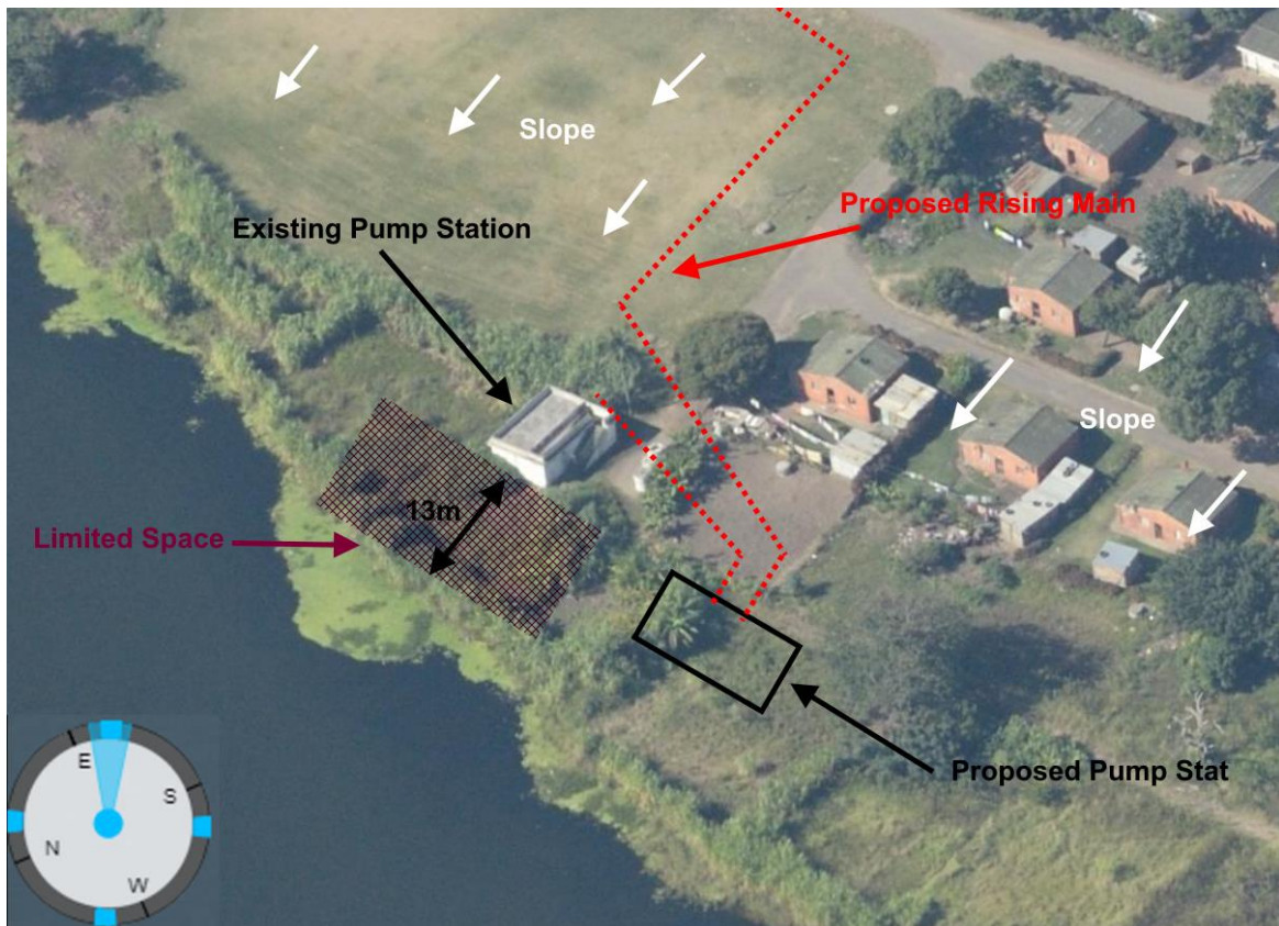
Figure 6: Oblique View of the Proposed Pump Station Site (Source: eThekweni Municipality, Oblique Viewer)
