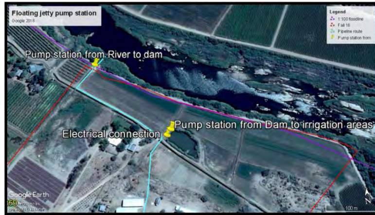
Figure 10: 1:100 Year flood line and pump station
