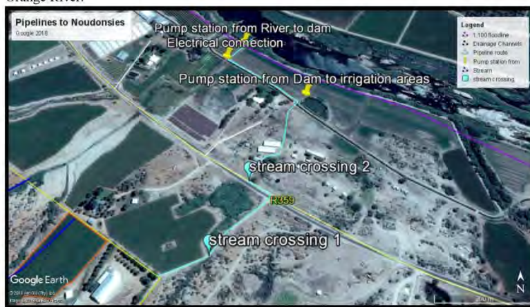
Figure 6: Pipelines from the pump station at the Orange River
