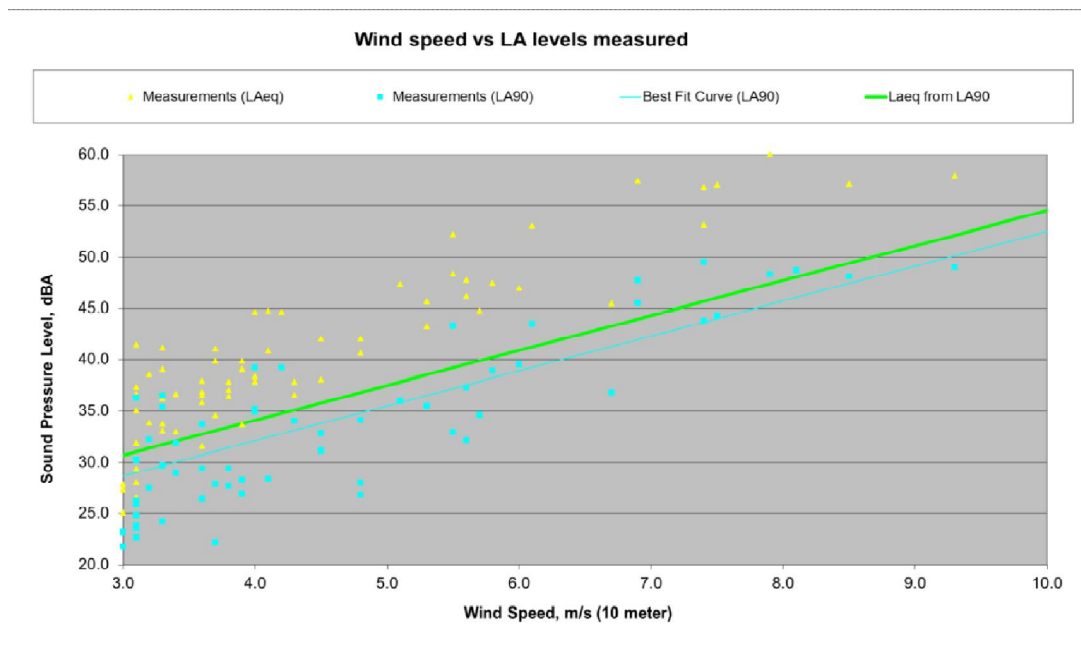
Figure 26: Ambient sound levels as wind speed increase
