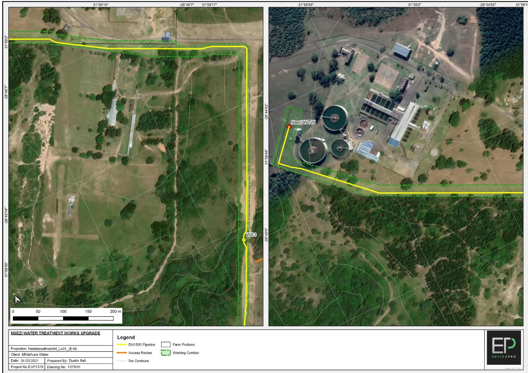
Figure 9: Aerial Photograph Showing Section 3 Of The DN1500 Pipeline Which Also Indicates The Working Corridor.
