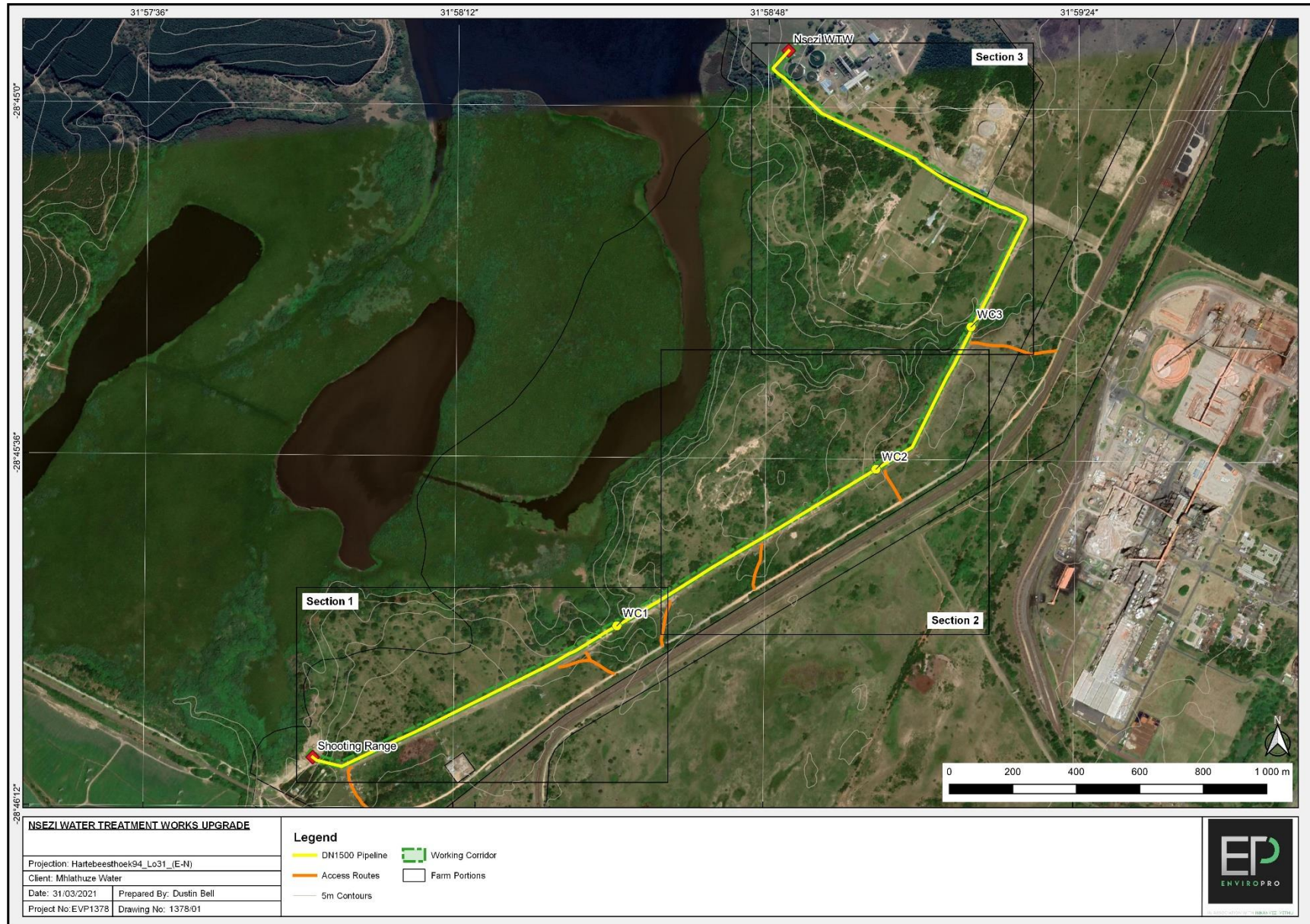
Figure 6: Aerial Photograph Showing The DN1500 Pipeline Which Also Indicates The Working Corridor.
