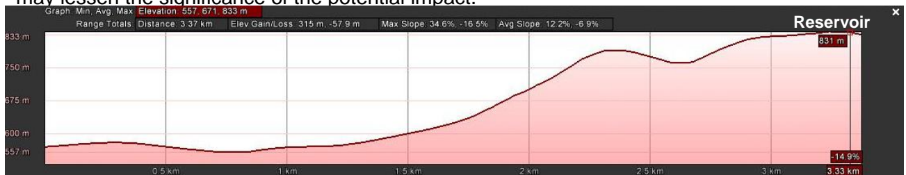
Figure 10: Elevation profile from Nkambeni Safari Camp to new reservoir over distance of 3 km
