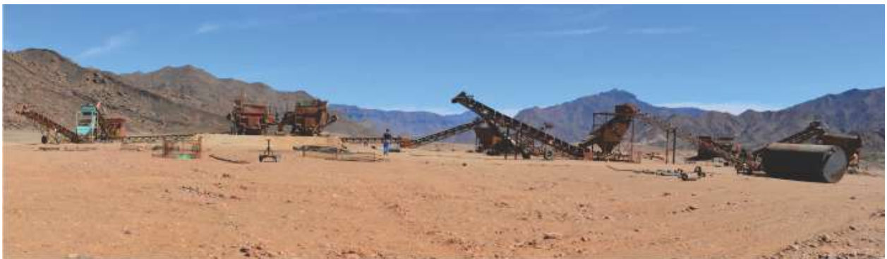
Photo 6: The recently established plant at Blokwerf with 1 x 16ft pan at present
