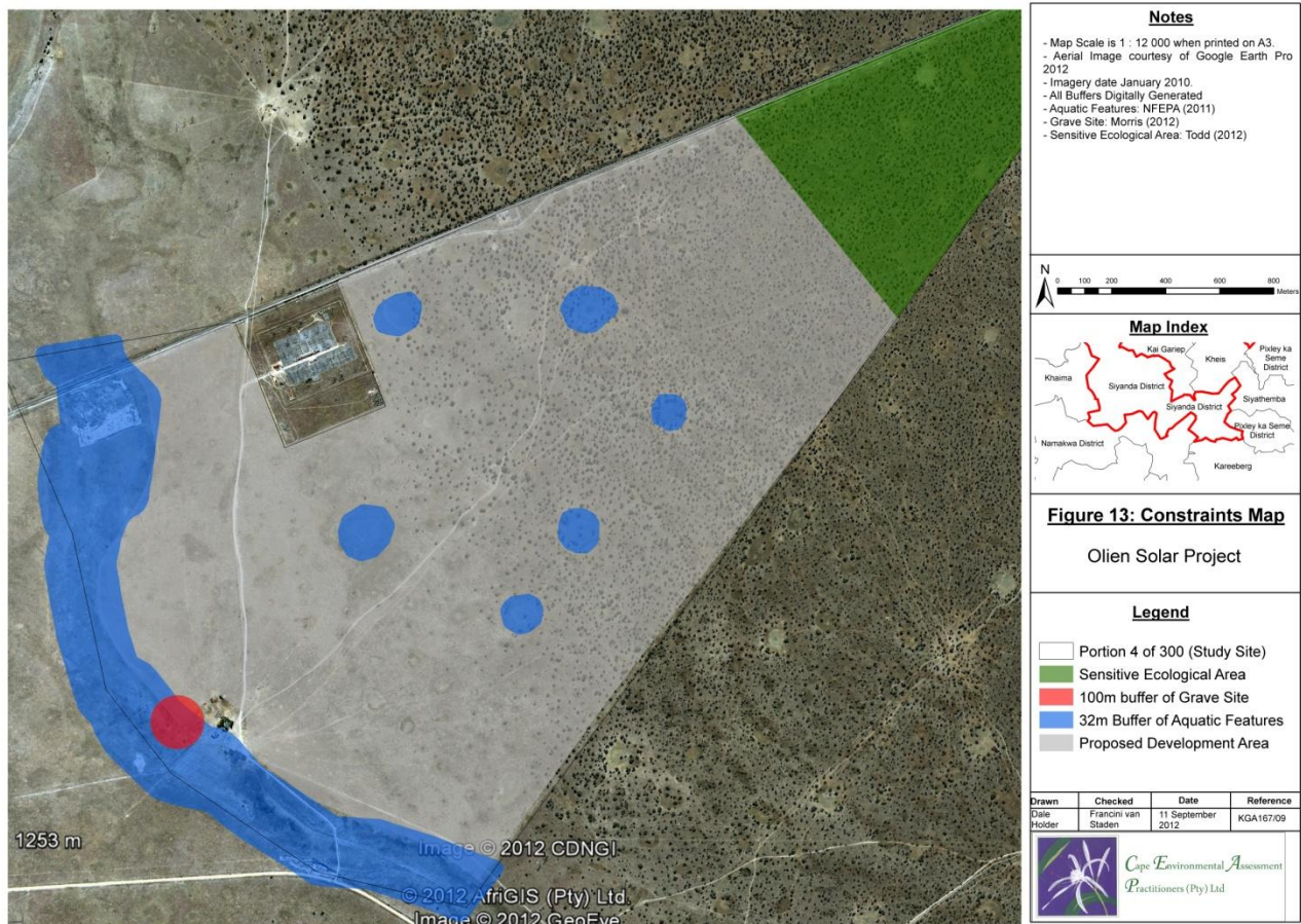
Figure 4: Site constraints map showing drainage line with 32-metre buffer, flat pans on development site with 32-metre buffers around these features, graves with 100-metre buffer and sensitive ecological north-eastern corner (See Appendix B for larger map).
