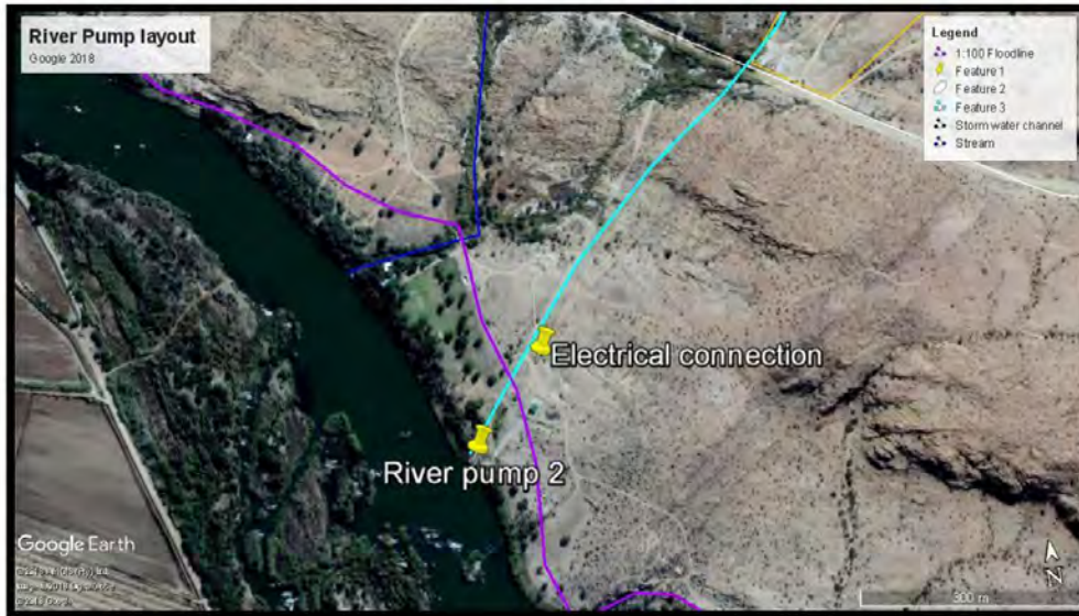
Figure 9: 1:100 Year flood line and pump station
