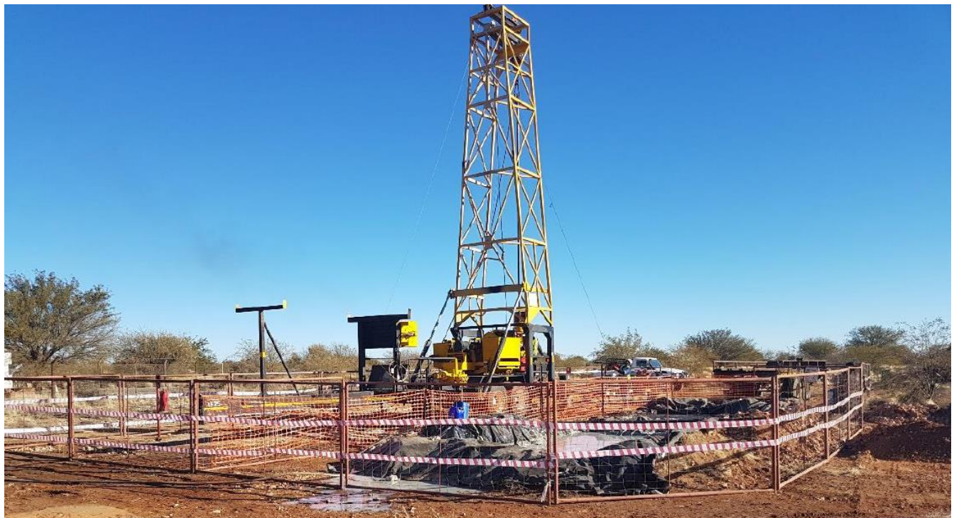
FIGURE 3-1: TYPICAL DIAMOND-CORE DRILLING RIG
