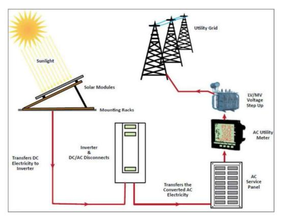
Figure 1:Overview of the solar power plant
